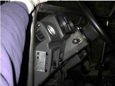
Remove the passenger side window defrost vent.
